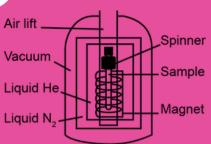
Sample is lowered into a magnet where it is spun and hit with electromagnetic pulses in the radio frequency (RF) range. The RF frequency is tuned to the specific nucleus you are studying (e.g. H-1 or C-13).
