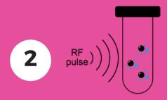
Nuclei absorb energy from the pulse and go from a lower energy state to a higher energy state.
